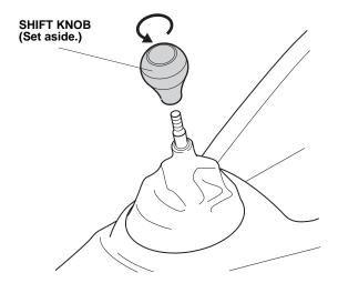
2. Install the new shift knob by turning it clockwise. Turn the knob until the orientation of the shift pattern is correct. The knob should turn 10 to 14 times.
