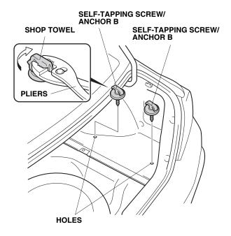
26. Repeat step 25 to install two self-tapping screws/ anchors B on the left side of the vehicle.
