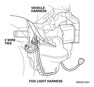
31. Secure the fog light harness to the vehicle harness with two wire ties as shown. Do not secure the fog light harness to the SRS harness.
