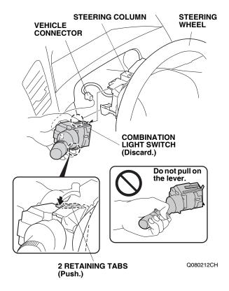
58. While pushing the two retaining tabs, slide the combination light switch out and remove it from the steering column.
