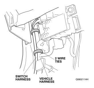
57. Unplug the vehicle connector from the combination light switch.
