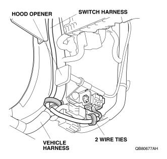
56. Secure the switch harness to the vehicle harness with two wire ties.
