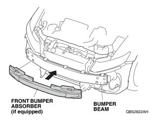
40. Plug the fog light harness 2-pin connector into each fog light, and with the help of an assistant, reinstall the front bumper.
