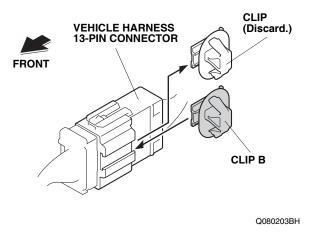
44. Unplug the vehicle harness 13-pin connector.
