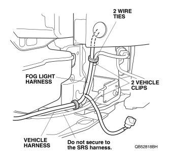
34. Route the fog light harness along the bumper beam as shown.
