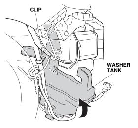
30. Secure the fog light harness to the vehicle harness with two wire ties. Do not secure the fog light harness to the washer tube.
