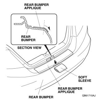
12. Use the soft sleeve to adhere the rear bumper applique to the lower section as shown.
