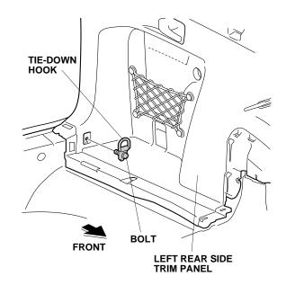
17. Pull away the weatherstrip from around the left rear side trim panel at the tailgate, and remove the door opening seal at the left rear door. Starting at the front, release the left rear side trim panel (eight clips and seven retaining tabs).
