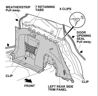
18. Release the wire and remove the left rear seat release lever (two clips and five retaining tabs), then remove the left rear side trim panel.
