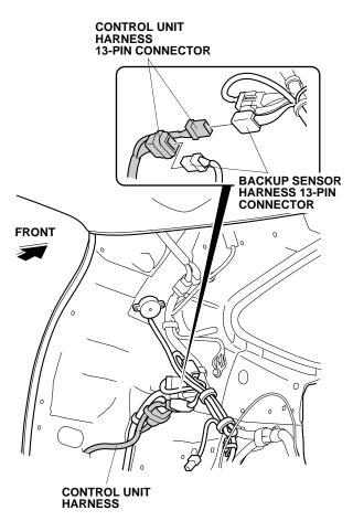
59. Plug the vehicle 13-pin connector into the control unit harness 13-pin connector. Go to step 61.
