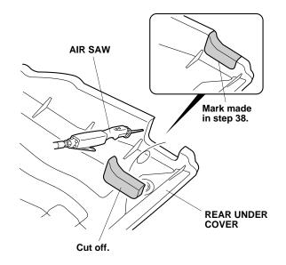
40. Using an air saw, cut the rear under cover along the scribe line as shown. Remove any burrs and sharp edges from the corners.
