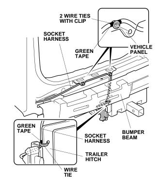
43. At the first green tape, secure the socket harness to the trailer hitch with one wire tie. At the next two green tapes, secure the socket harness to the vehicle panel with two wire ties with clip. 44. Route the socket harness as shown, and secure it to the hole in the bumper beam with one wire tie.
