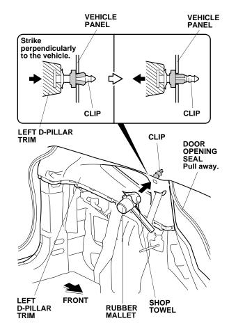
20. Using a rubber mallet wrapped with a shop towel, lightly tap the area marked "SIDE CURTAIN AIRBAG" on the left D-pillar trim to push in the clip. Make sure to strike area perpendicularly to the vehicle. 21. Remove the left D-pillar trim (ten clips).
