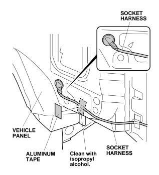
48. Inside the vehicle, secure the socket harness.2WD vehicle: Route the socket harness as shown, and secure it to the vehicle panel with one wire tie.
