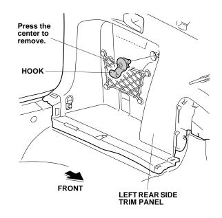
16. Remove the tie-down hook (one bolt).
