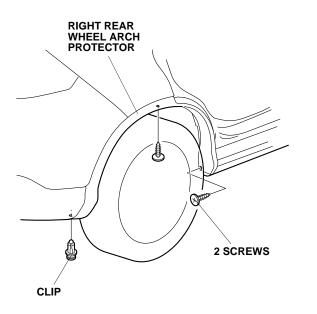
23. Remove the one clip and the two screws from the right rear wheel arch protector. If equipped, remove the splash guards.
