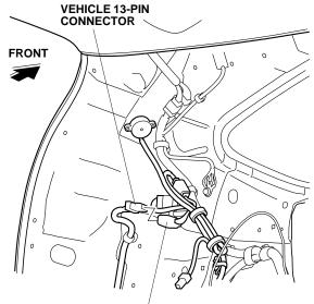
BACKUP SENSOR HARNESS 13-PIN CONNECTOR 58. Plug the control unit harness 13-pin connector into the backup sensor harness 13-pin connector.
