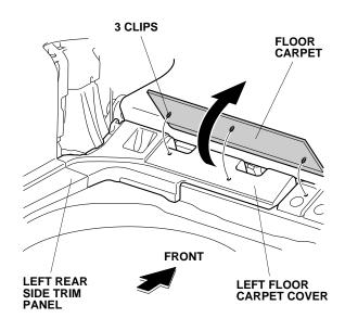
12. Remove the left floor carpet cover (three clips and two retaining tabs).
