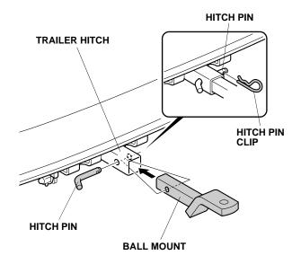
After the first 600 miles (1,000 km) of towing, have your Honda Dealer re-check the tightness of the trailer hitch bolts.
