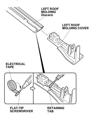
13. Reinstall the left roof molding cover in its original position on the roof.
