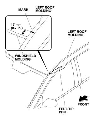
Using a plastic trim tool, pry up on the left roof molding cover to release one retaining tab and one clip.
