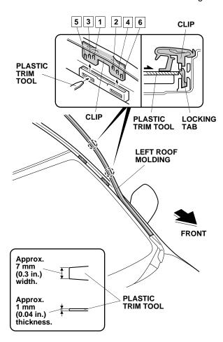
5. Place a blanket over the roof of vehicle under the left roof molding. Be careful not to deform the roof molding when measuring and cutting.
