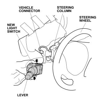
60. Plug the vehicle connector into the new light switch.
