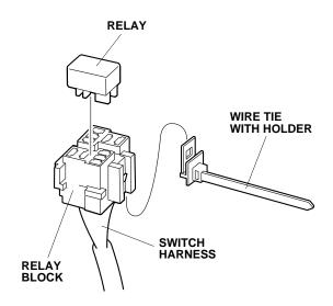
46. Install the wire tie with holder onto the switch harness relay block.
