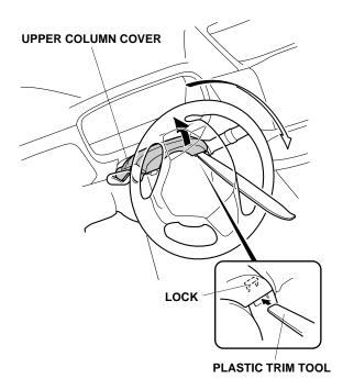
9. Secure the upper column cover to the meter panel with tape.
