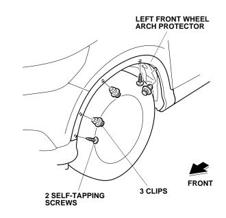
15. Remove the left front wheel arch protector (eight clips and three retaining tabs).
