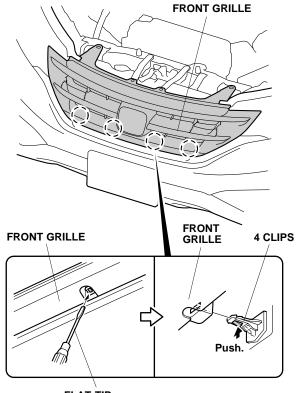
FLAT-TIP SCREWDRIVER 21. Using a long shank flat-tip screwdriver, release the one clip and two retaining tabs.
