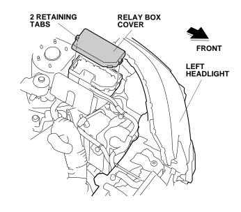
64. Using isopropyl alcohol on a shop towel, thoroughly clean the area where the fuse label will attach. Attach the fuse label to the relay box cover.
