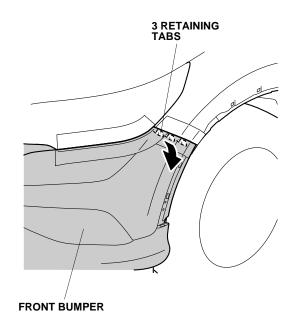
• Release the four retaining tabs on each side.
