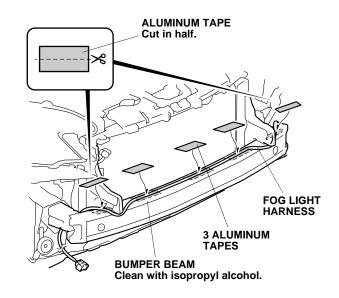
39. Cut one aluminum tape in half. Secure the fog light harness to the bumper beam with the two halves of aluminum tape.
