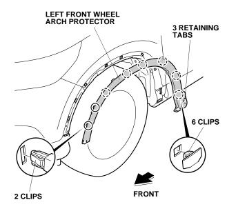
16. Repeat steps 14 and 15 to remove the front wheel arch protector from the right side of the vehicle.
