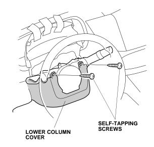
11. Remove the lower column cover (one self-tapping screw).
