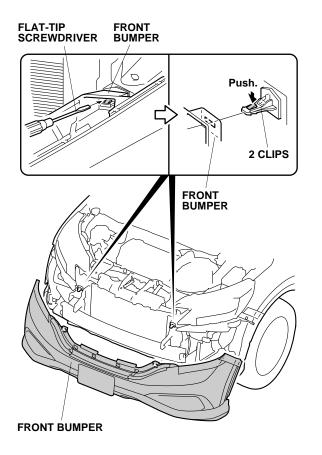
• With the help of an assistant, remove the front bumper. Place the front bumper on a blanket.
