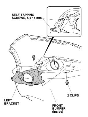
Install the fog light to the front bumper with two 5 x 14 mm self-tapping screws.
