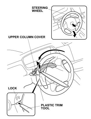
7. Using a plastic trim tool, release the lock as shown.
