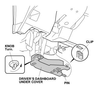
4. Remove the driver's dashboard lower cover (eight clips and unplug the vehicle connector).
