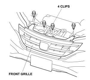
20. Using a flat-tip screwdriver, release the front grille (four clips).
