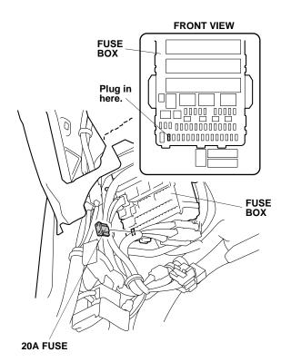
62. Using isopropyl alcohol on a shop towel, thoroughly clean the area where the fuse label will attach. Attach the fuse label to the fuse box label on the driver's dashboard under cover.
