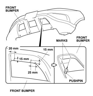
49. While wearing eye protection, drill both pierced marks using a 3 mm drill bit.
