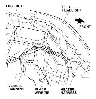
47. Across the top of the engine, secure the heater harness to the vehicle harness with five black wire ties.
