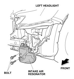
33. Remove the air intake tube (two bolts).
