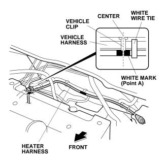
41. Align the mark at the point B with the vehicle clip, and secure the heater harness to the vehicle harness with three white wire ties and one black wire tie as shown.
