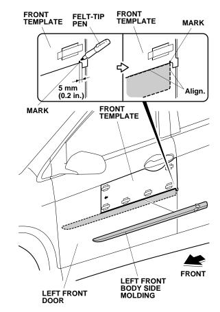
7. Align the left front body side molding with the front template and the mark you made on the front template, and attach it to the left front door as shown.
