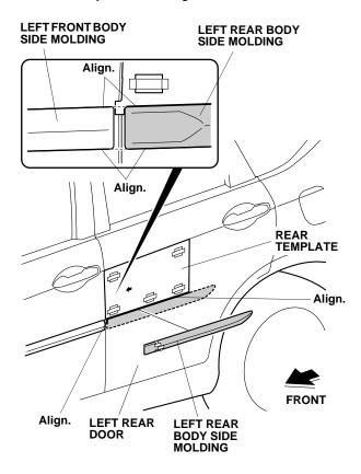
17. Press the left rear body side molding firmly with the palm of your hand and remove the adhesive backing 50 to 100 mm (2 to 4 in.) at a time.
