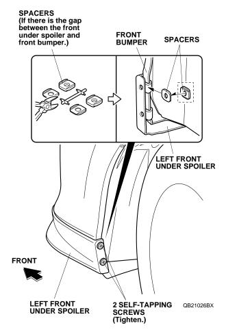
Turn the template over and repeat steps 2 through 17 to install the right front under spoiler on the right side of the vehicle.
