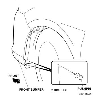
7. Thread a self-tapping screw into each pierced mark to make a hole in the front bumper. Remove the self-tapping screw.
