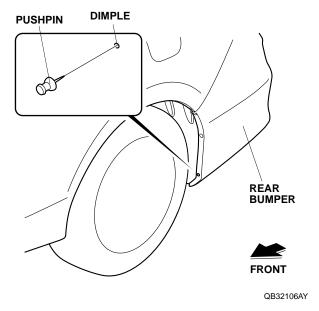
9. Gently pull away the rear bumper in the area shown. Using a felt-tip pen, mark the left rear inner fender at the measurement shown.
