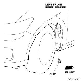
4. Install the left front splash guard to the left front inner fender with two washer-screws and the clip removed in step 3. Install them in this order 1→2→3. Make sure there is no gap between the left front splash guard and the vehicle body. If there is a gap, loosen the two washer-screws, hold the splash guard against the body, and retighten the washer-screws.
