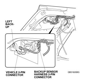
27. Plug the backup sensor harness 2-pin connector into the left backup light.
