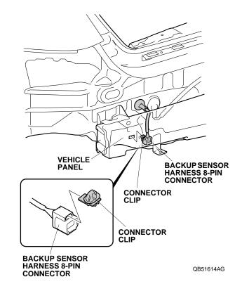
41. With the help of an assistant, bring the rear bumper next to the rear of the vehicle, plug the subharness8-pin connector into the backup sensor harness8-pin connector, and reinstall the rear bumper.
