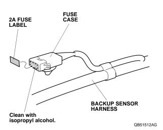
20. Secure the backup sensor harness to the vehicle harness with one wire tie.
