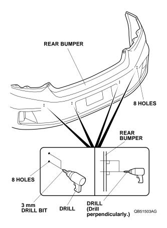
Using a 24 mm hole saw, enlarge the outboard (left and right corner sensor) bumper holes by drilling the upper 3 mm holes. Remove any burrs.
