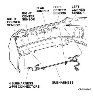
14. Secure the two subharness clips to the left sensor clip and right sensor clip as shown.
