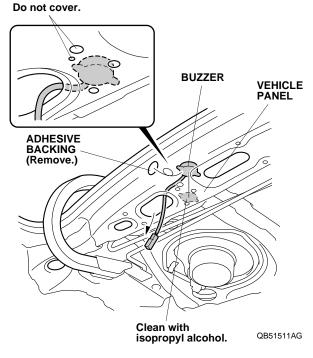
Remove the adhesive backing from the buzzer and attach it to the vehicle panel.
