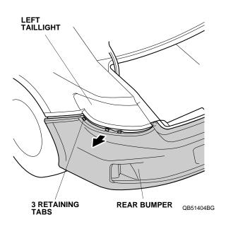
With the help of an assistant, unplug the vehicle connectors, remove the rear bumper (four retaining tabs).
