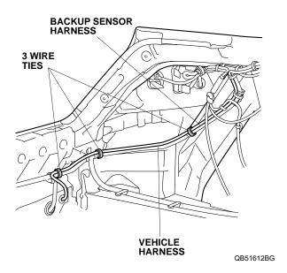
39. If equipped with vehicle harness, install the wire tie with holder to the backup sensor harness 8-pin connector, and secure it to the vehicle harness. Go to step 41.
