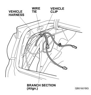
21. Secure the clip on the backup sensor harness to the vehicle panel.
