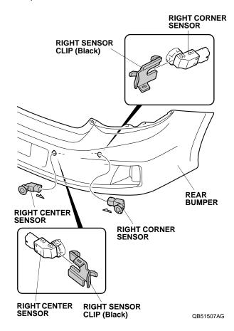
13. Plug the four subharness 2-pin connectors into the left center sensor, left corner sensor, right center sensor, and right corner sensor.
