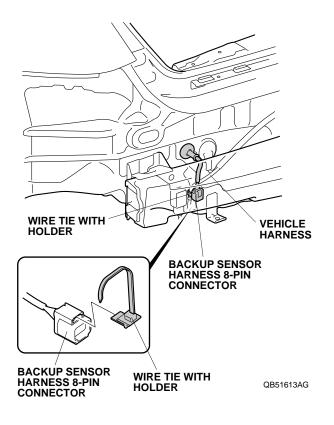
40. Install the connector clip to the backup sensor harness 8-pin connector, and secure it to the vehicle panel.
