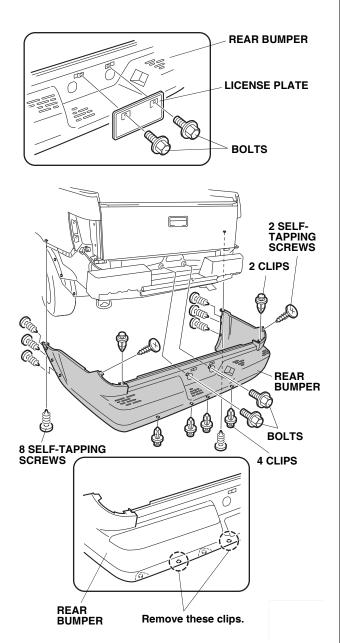
20. Remove the rear bumper (two bolts, ten self-tapping screws, and six clips). Have an assistant help you when removing the rear bumper. Place the rear bumper on a blanket.
