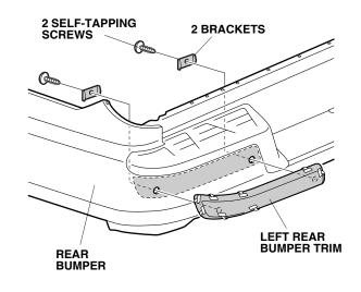
26. While applying light pressure against the left rear bumper trim, carefully remove the taped adhesive backings.
