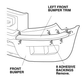
12. Using the palm of your hand, firmly press the left front bumper trim against the front bumper.
