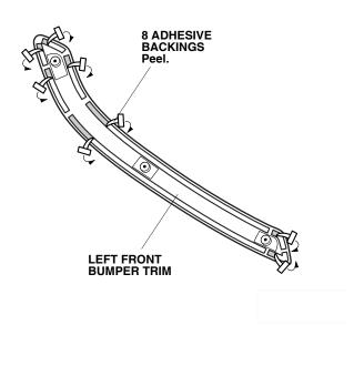
10. Align the left front bumper trim to the front bumper and loosely secure it with three brackets and three self-tapping screws.
