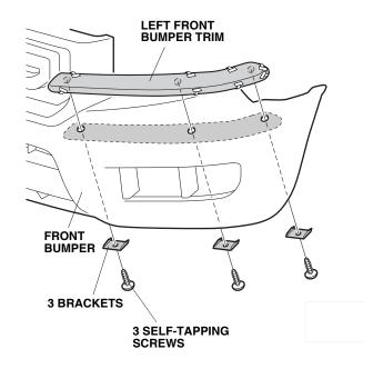
11. While applying light pressure against the left front bumper trim, carefully remove the taped adhesive backings.
