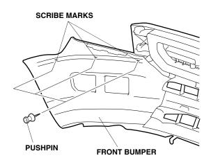
7. While wearing eye protection, drill 3 mm holes at the three marks made in step 6, then enlarge the holes with a 30 mm hole saw. Remove any burrs.
