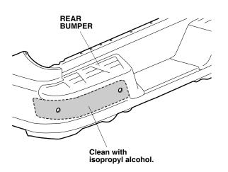
24. Attach masking tape to the ends of the adhesive backings on the left rear bumper trim. Peel the adhesive backings partway and attach them to the front surface of the left rear bumper trim.
