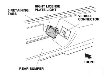
19. Remove the license plate from the rear bumper (two bolts).
