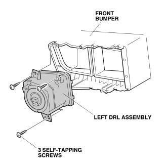
6. Using a pushpin, locate and pierce three scribe marks on the inside of the front bumper.
