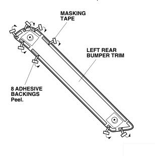
25. Align the left rear bumper trim to the rear bumper and loosely secure it with two brackets and two self-tapping screws.
