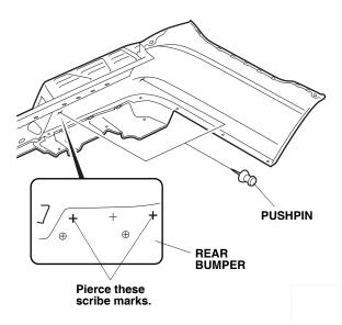
22. While wearing eye protection, drill 3 mm holes at the two marks made in step 21, then enlarge the holes with a 30 mm hole saw. Remove any burrs.
