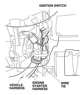
56. Adjust the steering wheel in, out, up, and down while you check the engine starter harness routing. If the harness is rubbing against the steering column bracket, check the installation and position of the wire ties installed in steps 53 and 55.
