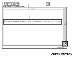
10. Input the PCM code, then click the check button. NOTE: To ensure security, the PCM code (password) is changed everyday, so it is impossible to register the remote control engine starter if the dates of the PCM code acquisition and registration are different. The date of the HDS tester should also match.
