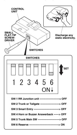
Check the settings of the switches on the control unit.
