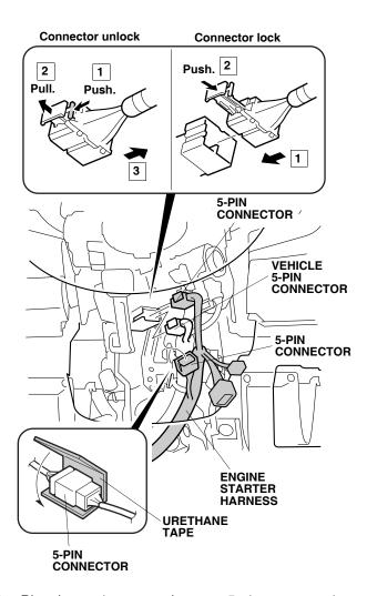
51. Plug the engine starter harness 5-pin connector into the vehicle 5-pin connector.
