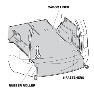
8. Align the cargo liner to the right rear side panel. Fold the cargo liner back and, using two alcohol swabs, thoroughly clean the area where the fasteners will attach. After cleaning with the alcohol swabs, wait at least 3 minutes before continuing to the next step.
