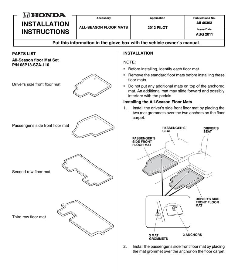
3. Install the second row floor mat by placing the two mat grommets over the two anchors on the floor carpet.
