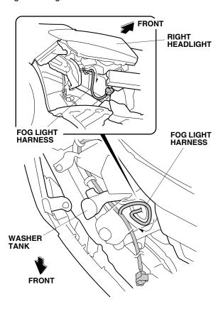
17. Install one wire tie with clip to the fog light harness at the green tape. Install the wire tie with clip into the vehicle panel hole.
