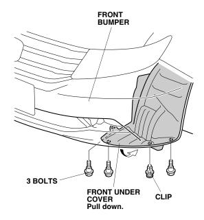
2. Insert your hand behind the under cover, and unplug the vehicle connector from the left fog light. Remove the bulb by turning it counterclockwise.
