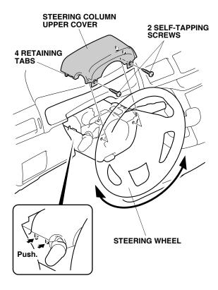
31. Remove the steering column upper cover (two self-tapping screws and four retaining tabs). Turn the steering wheel (right or left) to access each self-tapping screw.
