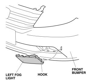
27. Secure the left fog light to the front bumper with one 5 x 16 mm washer-bolt.
