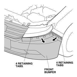
Remove four self-tapping screws, eight bolts, and four clips from the front bumper.
