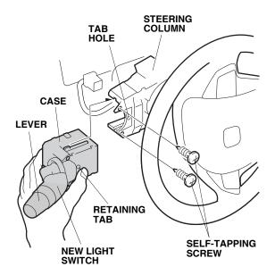
36. Plug the light switch connector into the new light switch.
