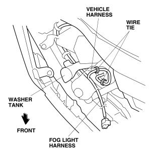
Route the fog light harness along the vehicle harness, and secure it to the vehicle harness with six wire ties.
