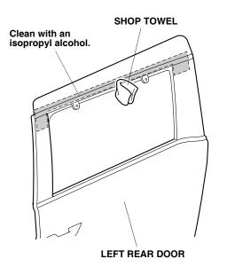
15. Peel back 1½ to 2 inches of each adhesive backing, and tape the ends to the front surface of the left rear door visor with masking tape.
