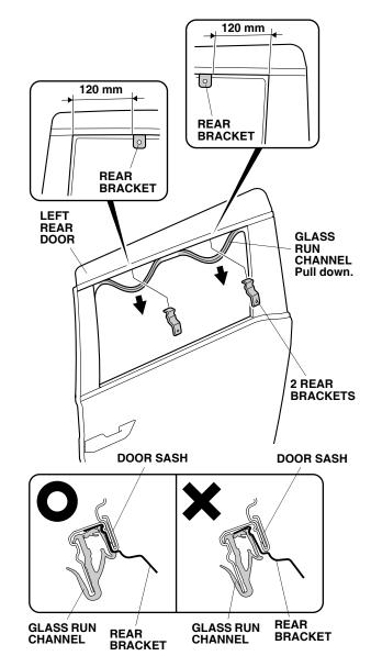
13. Reinstall the glass run channel to secure the two rear brackets. Be sure the brackets are installed tightly to the door sash, and that the glass run channel is properly seated.
