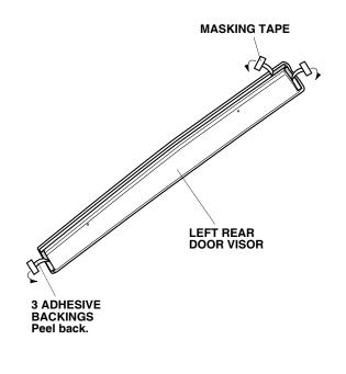
16. Place the door visor against the door, and adjust the visor so it lines up with the two rear brackets.
