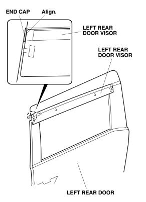
While applying light pressure against the left rear door visor, carefully remove the adhesive backings. Push up on the rear brackets while removing the adhesive backings.
