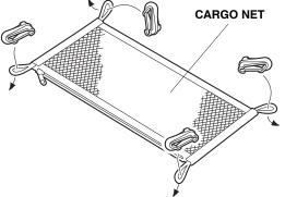
2. Position the cargo net with the zipper facing the rear of the vehicle. Attach the four cargo net hooks to the four tie-down rings.
