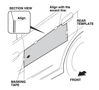
9. Peel back approximately 1½ to 2 inches of the adhesive backing, and tape the ends to the outer surface of the body side molding. Remove the small end pieces of adhesive backing.
