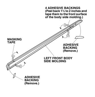
3. Clean the location where the left front body side molding will attach with one alcohol swab.
