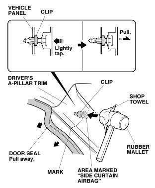
12. Using a rubber mallet wrapped with a shop towel, tap lightly on the area marked "SIDE CURTAIN AIRBAG" on the driver's A-pillar trim to push in the clip. Make sure to tap perpendicular to the A-pillar surface.
