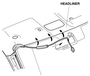
AUTOMATIC DAY/NIGHT MIRROR HARNESS 29. Plug the automatic day/night mirror harness 7-pin connector into the automatic day/night mirror.
