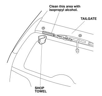
26. Remove the adhesive backing from the hook and loop fastener, and attach it to the tailgate at the end of the template.
