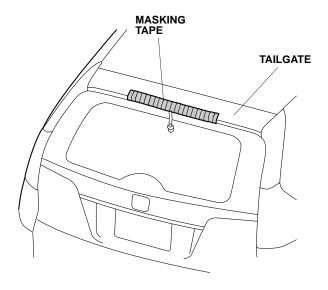
7. Place template B on the top right corner of the tailgate, and align it to the edge of the tailgate. Secure the template in place with masking tape.
