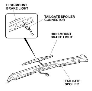
36. Install the high-mount brake light onto the tailgate spoiler using two flange nuts. Torque the two flange nuts to 5.0 N·m (3.7 lbf·ft).
