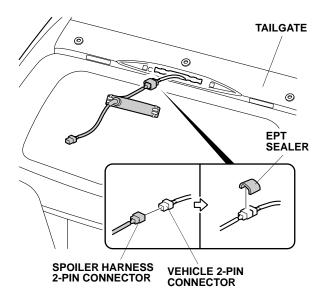
32. Install the spoiler harness on the tailgate, and remove the four adhesive backings.
