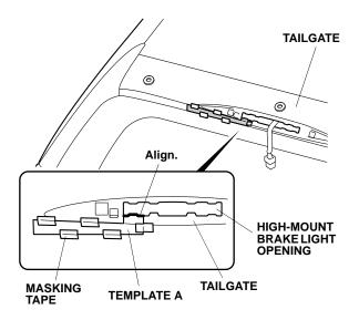
25. At the left end of the template, use isopropyl alcohol on a shop towel to clean the tailgate where the hook and loop fastener will attach.
