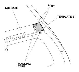
8. Using a felt-tip pen, mark the tailgate through the hole in template B.
