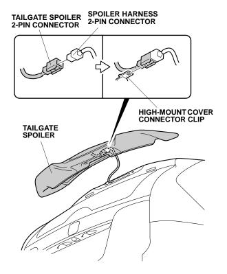
39. Attach the 2-pin connector to the high-mount cover connector clip.
