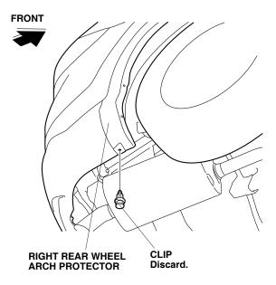
12. Using a pushpin, pierce the center of inner clip on the right rear inner fender.
