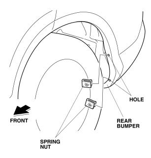
Install the left rear splash guard to the rear bumper with two washer-screws in the order 1→2.
