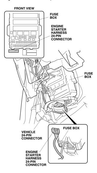
67. Secure the engine starter harness to the vehicle harness with two wire ties.
