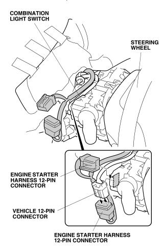
81. Plug the remaining engine starter harness 12-pin connector into the combination light switch.
