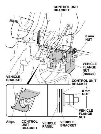
92. Install the control unit bracket on top of the vehicle bracket and align the control unit bracket with the edge of the vehicle bracket. Reinstall the vehicle flange nut. Install the 8 mm nut (supplied) on top of the vehicle flange nut.
