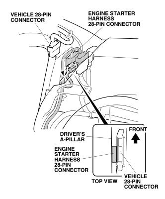
46. Plug the vehicle 28-pin connector into the engine starter harness 28-pin connector.
