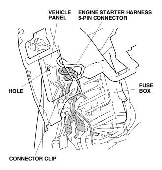
52. Slide the other clip on the engine starter harness onto the vehicle connector. Note the direction and the orientation of the clip.
