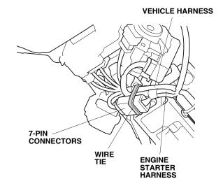
76. Route the engine starter harness across the steering column area as shown.
