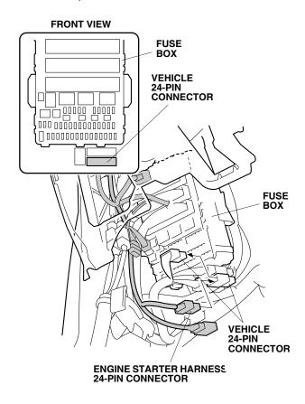
66. Slide the clip from the engine starter harness 24-pin connector onto the bottom of the fuse box, then plug the remaining vehicle 24-pin connector into the engine starter harness 24-pin connector.
