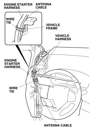
48. Secure the engine starter harness and the antenna cable to the vehicle harness with one wire tie.
