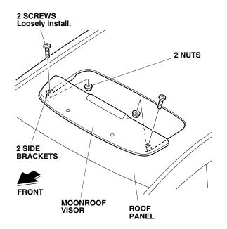
14. Position the moonroof visor with equal spacing on each sides. Check that the rubber molding is not twisted or rolled under the visor.
