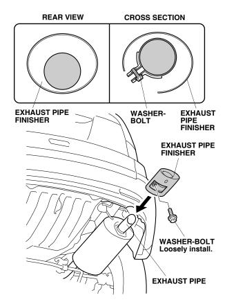
2. Continue to slide the exhaust pipe finisher in until it contacts the end of the exhaust pipe. While holding the exhaust pipe finisher firmly against the exhaust pipe, torque the washer bolt to 10 N·m (7 lbf·ft).
