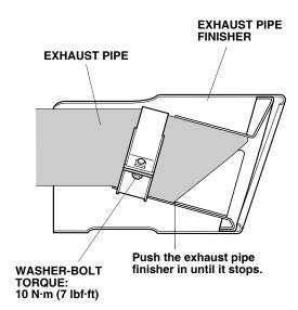
3. Start the engine, and rev it up a few times. Listen for vibration from the exhaust pipe finisher, and adjust if necessary.
