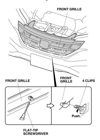
12. Using a long blade flat-tip screwdriver, release the one clip and the two retaining tabs from each side of the front grille.
