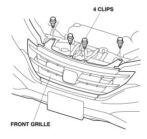
11. Using a flat-tip screwdriver, release the 4 clips from the bottom of the front grille.
