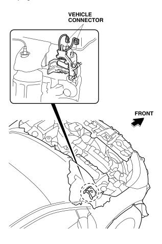
35. Release the vehicle harness holder from the vehicle bracket (two hooks).
