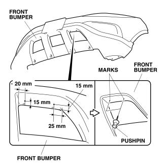
49. While wearing eye protection, drill both pierced marks using a 3 mm drill bit.
