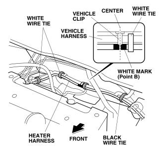
42. Route the heater harness to the driver's side of the fuse box as shown.
