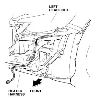
45. Align the mark at point C and D with the vehicle clip, and secure the heater harness to the vehicle harness with five black wire ties as shown.
