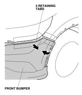
Attach masking tape to the front bumper in the area shown.
