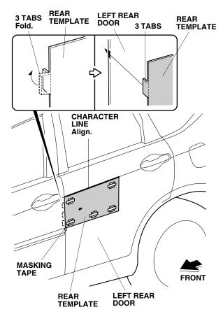
Align the rear template with the character line, and attach it to the left rear door using strips of masking tape. 15. Peel back about 40 to 50 mm (1½ to 2 in.) of adhesive backing from each adhesive tape, and tape the ends to the front surface of the left rear body side molding. Remove the other adhesive backings.
