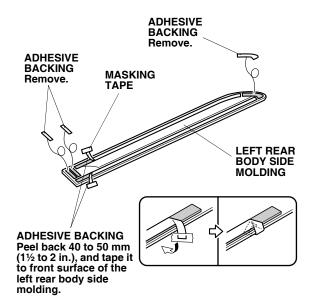
16. Align the edges of the left rear body side molding with the edges of the rear template, and install the left rear body side molding on the left rear door.
