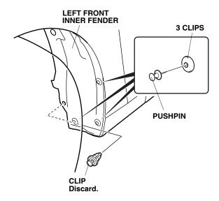
3. Using a pushpin, make small holes through the centers of the three clips shown.
