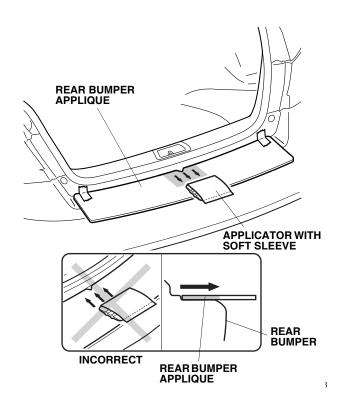
Starting at the center and working outward, use the applicator to smooth the rear bumper applique.
