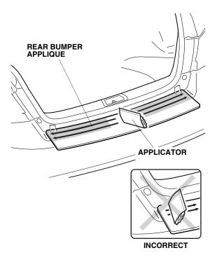
11. Once the upper surface is completely smooth with no bubbles, use the applicator to apply the rear bumper applique to the rounded rear edge at the center as shown.
