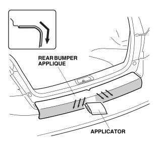
13. Remove the protective film from the rear bumper applique. Remove the protective film slowly; do not pull up the protective film.
