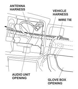
22. Route the antenna harness as shown and secure it to the vehicle harness with two loosely-installed wire ties.
