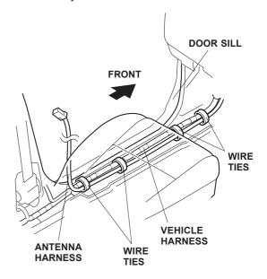
25. Get the bus cable. Route the antenna harness and the bus cable under the floor carpet and pull them out of the cutout in the floor carpet.
