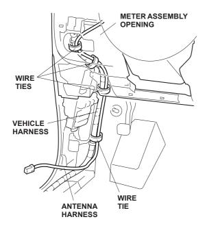
24. Route the antenna harness as shown and temporarily secure it to the vehicle harness with four loosely-installed wire ties.
