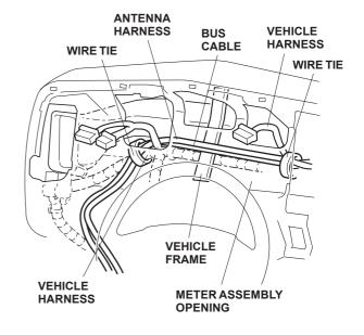
37. Align the end of the bus cable connector with the end of the vehicle 20-pin connector and secure the bus cable to the vehicle harness using a wire tie.
