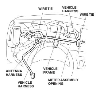
23. Route the antenna harness along the vehicle harness and temporarily secure it to the vehicle harness with four loosely-installed wire ties.
