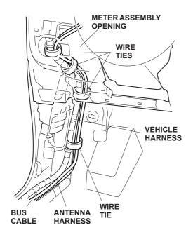
36. Route the bus cable as shown. Secure the bus cable and antenna harness to the vehicle harness by tightening the two wire ties loosely-installed in step 22.
