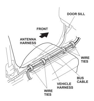
35. Route the bus cable along the antenna harness as shown. Secure them to the vehicle harness by tightening the four wire ties loosely-installed in step 23.
