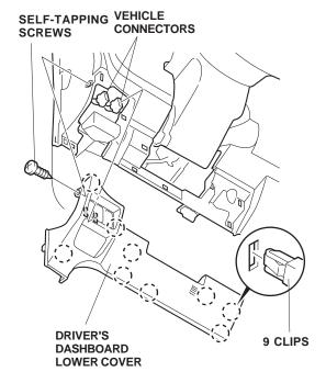
Using a tape measure and felt-tip pen, measure and mark the driver's dashboard lower cover.
