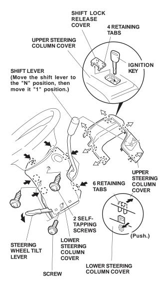
10. Using a tape measure and felt-tip pen, measure and mark the steering column upper cover.
