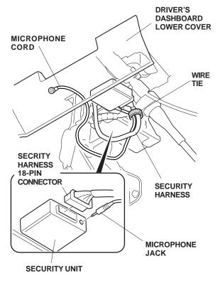
28. Fold the security harness and microphone wire, and secure then with one wire tie so that there is no tension applied to the microphone jack.
