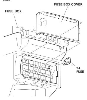
31. Attach the fuse label (OPTION FUSE 2A) over the No.33 slot on the inside of the fuse box cover.
