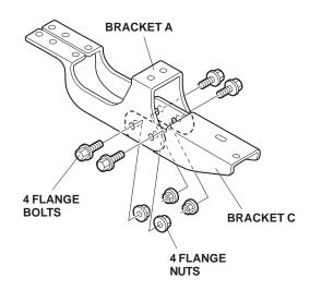
Assemble two rear bracket assemblies using brackets B and C along with four flange bolts and four flange nuts. Leave the nuts and bolts loose at this time.
