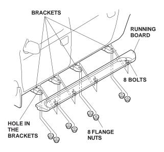
11. Align the rear of the running board with the end of the inner fender, then tighten the flange bolts you installed in step 9. Torque 14 flange bolts to 27 N·m (20 lbf·ft) and the one remaining flange bolt to 7 N·m (5 lbf·ft).
