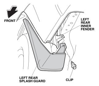
4. Install the left rear splash guard with two self-tapping screws in the order shown. Make sure that there is no space between the rear bumper and the splash guard before tightening the screws.
