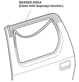
13. Attach strips of masking tape to the ends of the long adhesive backings, and remove 2 to 3 in. (5 to 8 cm) of adhesive backings. Fold back the ends, and tape the ends to the front of the door visor. Remove the short adhesive backing.
