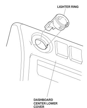
10. Align the locating tab on the socket with the cutout in the ring, and slide the cigarette lighter socket into the lighter ring. Push the cigarette lighter into the socket.
