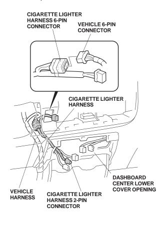
12. Connect the vehicle 2-pin connector and cigarette lighter harness 2-pin connector into the socket of the cigarette lighter. Reinstall the dashboard center lower cover.
