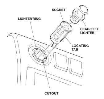
11. Route the cigarette lighter harness 2-pin connector along the vehicle harness and through the dashboard center lower cover opening. Plug the vehicle 6-pin connector into the cigarette lighter harness 6-pin connector.
