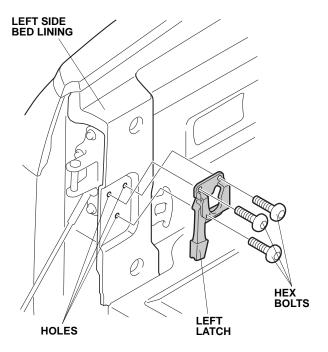
Install the left latch to the left side bed lining with three hex bolts. 3. Remove the left front lower tie-down hook (two T-50 torx bolts).
