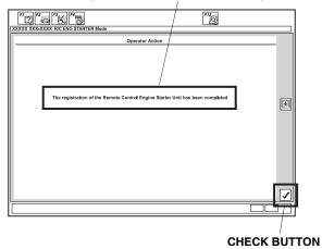
12. The following message will display: Check that the engine can be started by the Transmitter. Click on the check button.
