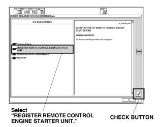
The following message will display: Obtain PCM-code (IMMOBILIZER PCM CODE) from iN. This vehicle's VIN will be required to obtain the password. (USA). Click on the check button.
