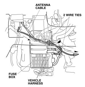
69. Route the antenna cable terminal toward the right side of the vehicle, and plug it into the control unit as shown.
