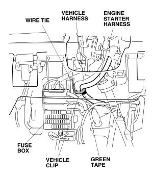
36. Locate and remove the blue tape from the vehicle 2-pin connectors (white), and unplug the vehicle 2-pin connectors as shown.
