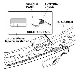
65. Clean the vehicle panel surface where the urethane tape will attach with isopropyl alcohol. Secure the antenna cable to the vehicle panel with the remaining part of the urethane tape you cut in step 40. Be careful not to crease the headliner.
