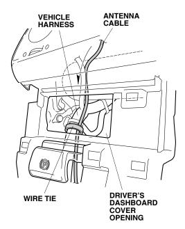
68. Route the antenna cable along the engine starter harness. Secure the antenna cable to the vehicle harness with the two wire ties that were secured loosely in step 44.
