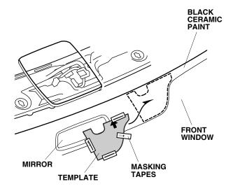
60. Using isopropyl alcohol on a shop towel, clean the area where the antenna will attach. Allow to dry before proceeding.
