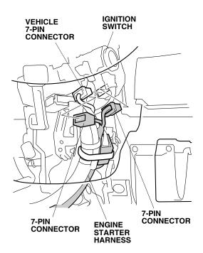
55. Secure the engine starter harness to the vehicle harness with one wire tie as shown.
