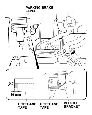
41. Clean the vehicle bracket surface with isopropyl alcohol where the urethane tape will attach. Attach the 10 mm piece of urethane tape that you cut in step 40 to the vehicle bracket as shown.
