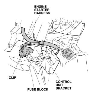
30. Install the engine starter harness clip on the vehicle bracket.
