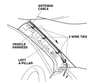
67. Secure the antenna cable to the vehicle harness with one wire tie.
