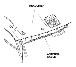
64. Clean the vehicle panel surface with isopropyl alcohol where the urethane tape will attach. Secure the antenna cable to the vehicle panel with one half of the urethane tape that you cut into two in step 40. Be careful not to crease the headliner.
