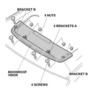
10. Adjust the position of the moonroof visor. Check that the brackets A and brackets B are firmly secured. Make sure the rubber molding on the moonroof visor is not twisted or rolled under the visor.
