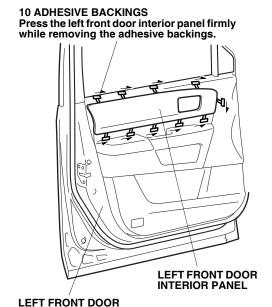
25. Using a rubber roller, apply pressure against the left front door interior panel and roll from one end to the other.
