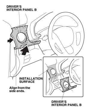
17. Press the driver's interior panel B firmly while removing the adhesive backings that you temporarily attached to the surface side.
