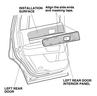
40. Press the left rear door interior panel firmly while removing the adhesive backings that you temporarily attached to the surface side.
