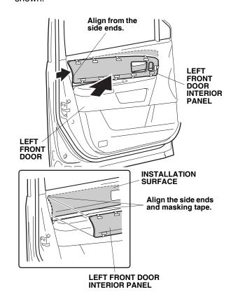
32. Press the left front door interior panel firmly while removing the adhesive backings that you temporarily attached to the outer surface.
