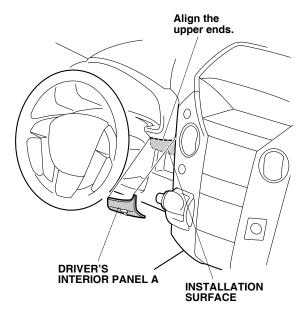
11. Press the driver's interior panel A firmly while removing the adhesive backing that you temporarily attached to the outer surface side.
