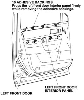
33. Using a rubber roller, apply pressure against the left front door interior panel and roll from one end to the other.
