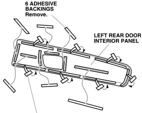
7 ADHESIVE BACKINGS Attach a piece of tape to an end. Peel back the adhesive backing partway and attach it to the outer surface of the panel.
