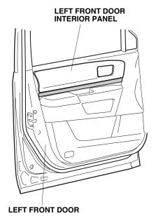
20. Using isopropyl alcohol on a shop towel, clean the area where the left front door interior panel will attach.
