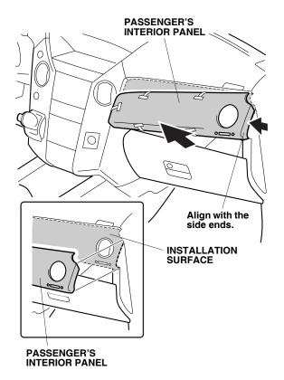
5. Press the passenger's interior panel firmly while removing the adhesive backings that you temporarily attached to the outer surface.
