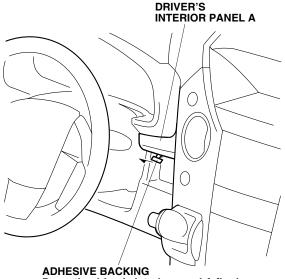
Press the driver's interior panel A firmly while removing the adhesive backing.
