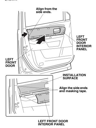
24. Press the left front door interior panel firmly while removing the adhesive backings that you temporarily attached to the outer surface side.
