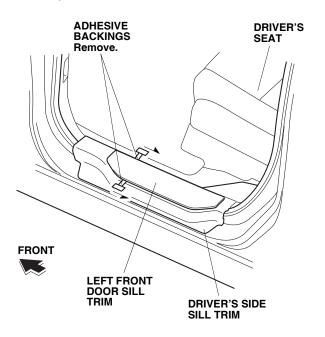
11. Using a rubber roller, apply pressure against the left front door sill trim and roll from one end to the other.
