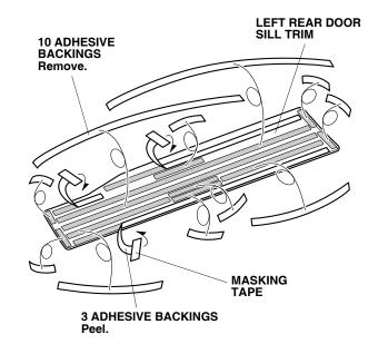
19. Remove the remaining adhesive backings.
