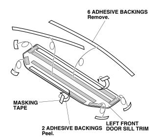
8. Remove the remaining adhesive backings.
