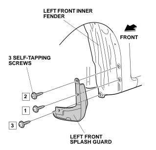
4. Turn the steering wheel all the way clockwise and repeat steps 1 thru 3 to install the right splash guard.
