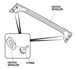
16. Using a utility knife, cut two slits in the two adhesive backings on the hatch spoiler.
