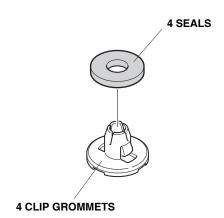
14. Install the four clip grommets into the four holes in the hatch. Press each clip until you hear a click.
