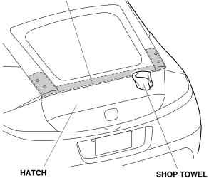
13. Install the four seals on the four clip grommets.
