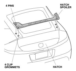
19. While applying light pressure to the hatch spoiler, carefully remove each adhesive backing in the order shown, while pushing the hatch spoiler against the hatch as shown.
