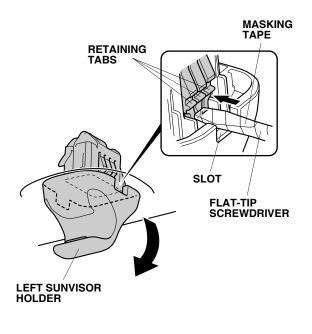
10. While holding down the sunvisor holder as shown, use a flat-tip screwdriver wrapped with masking tape to remove the left sunvisor holder (three retaining tabs).
