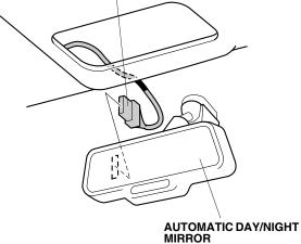
29. Align the green tape on the automatic day/night mirror harness at the headliner. Route the automatic day/night mirror harness through the grooves on the harness cover. Secure the harness cover to the mirror stay.
