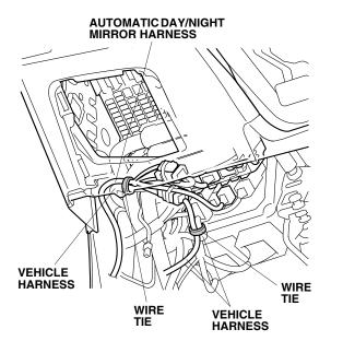
23. Secure the vehicle harness to the vehicle harness with one wire tie.
