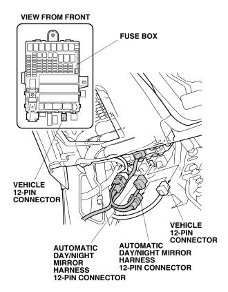
22. Secure the automatic day/night mirror harness to the vehicle harness with one wire tie.
