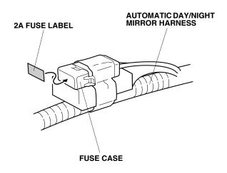
20. At the fuse box, unplug the vehicle 8-pin connector. Plug the automatic day/night mirror harness 8-pin connector into the fuse box 8-pin connector. Plug the vehicle 8-pin connector into the automatic day/night mirror harness 8-pin connector as shown.
