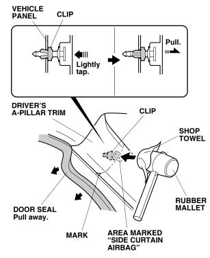
12. Using a rubber mallet wrapped with a shop towel, lightly tap the area marked "SIDE CURTAIN AIRBAG" on the top of the driver's A-pillar trim to push in the clip. Make sure to strike the area perpendicular to the vehicle. 13. Remove the driver's A-pillar trim (two clips).
