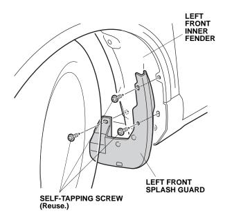
4. Turn the steering wheel all the way clockwise, and repeat steps 2 and 3 to install the right splash guard.
