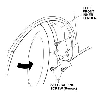
3. Position the left front splash guard on the left front inner fender, and install the three self-tapping screws you removed in step 2.
