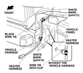
36. If there is no vehicle harness, secure the heater harness to the vehicle panel with two wire ties with clips (point C and point D).
