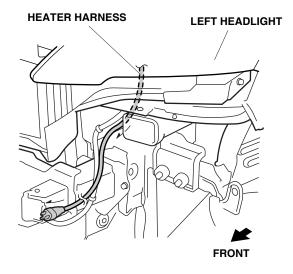
35. Secure the heater harness to the vehicle harness with two black wire ties (point C and point D).
