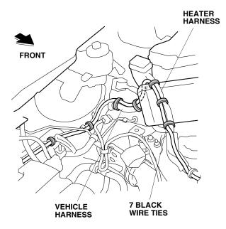
39. Secure the heater harness to the vehicle harness with two white wire ties and one black wire tie as shown.
