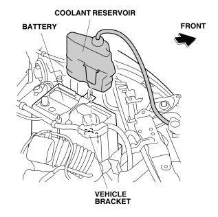
22. Remove the vehicle bracket (one vehicle bolt).
