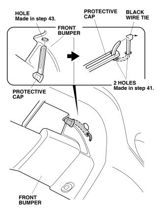
47. Secure the protective cap to the front bumper using one black wire tie as shown.
