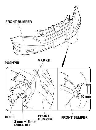
41. While wearing eye protection, drill the two pierced marks with a 3 mm drill bit and then enlarge the holes with a 5 mm drill bit.
