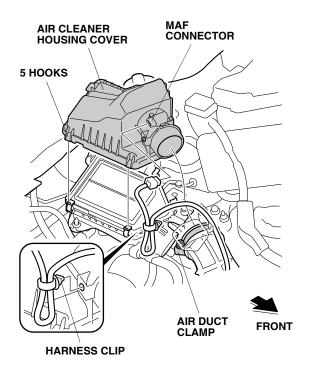
20. Remove the air cleaner housing (one bolt and two pins).
