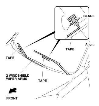
7. Remove the windshield wiper arms (two caps and two nuts). Wiper arm nut torque is 29.4 N·m (21.6 lbf·ft).
