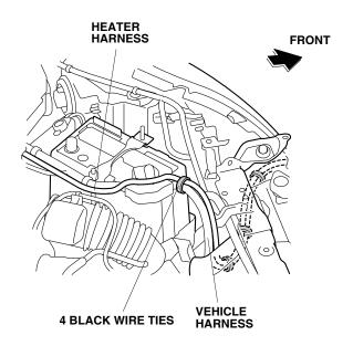
38. Secure the heater harness to the vehicle harness with seven black wire ties as shown.
