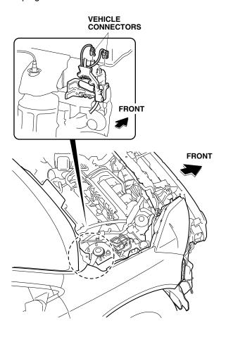
24. Release the vehicle harness holder from the vehicle bracket (two hooks).
