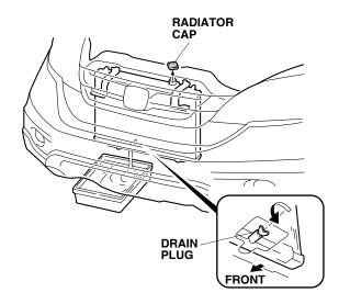
5. After the coolant drains completely, reinstall the radiator cap to prevent dust and dirt contamination.
