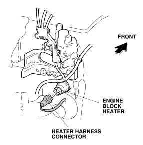
29. Secure the heater harness to the vehicle harness holder with a white wire tie (point A).
