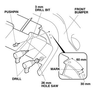
45. While wearing eye protection, drill the mark made in step 44 with a 3 mm drill bit, and then enlarge the hole with a 26 mm hole saw.
