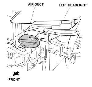
19. Loosen the air duct clamp. Remove the air cleaner housing cover (MAF connector, harness clip, and five hooks).
