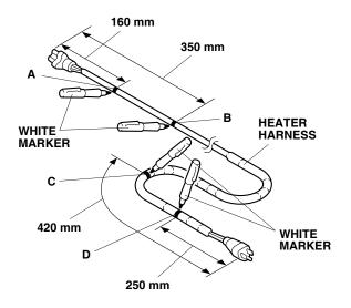
28. Plug the heater harness connector to the engine block heater.
