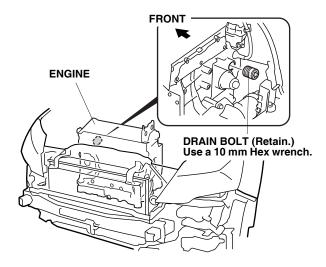
26. Install the engine block heater with aluminum washer into the bolt hole using a 24 mm socket and a torque wrench. Torque the engine block heater to 60 N·m (44 lbf·ft).
