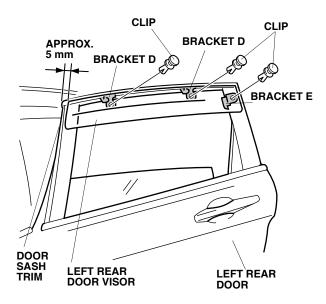
4. Attach masking tape to the left rear door at both ends of the door visor, then remove the left rear door visor (three clips).
