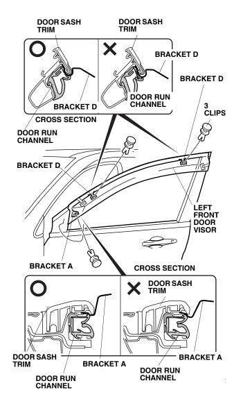
20. Using the palm of your hand, push up on the left front door visor while removing the two adhesive backings. Make sure there is no clearance between the brackets and the door sash trim.
