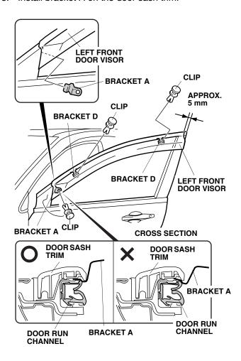
14. Position the left front door visor on the door sash by hooking the front bracket of the door visor on the door sash. Adjust the positions of bracket A and brackets D and install the three clips. Make sure there is no clearance between the brackets and the door sash trim. 15. Attach masking tape to the door sash at the ends of the left front door visor, then remove the door visor (three clips).
