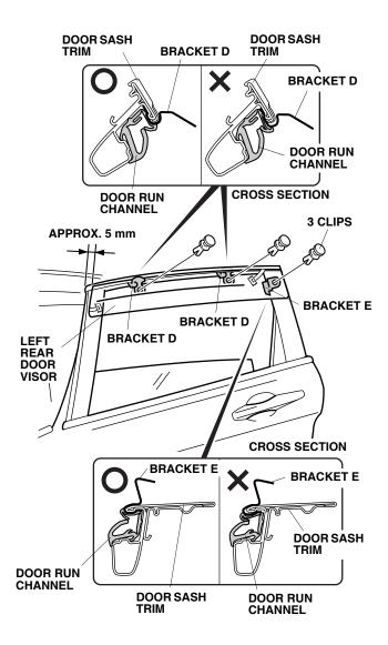
9. Using the palm of your hand, push up on the left rear door visor while removing the two adhesive backings. Make sure there is no clearance between the brackets the and door sash trim.
