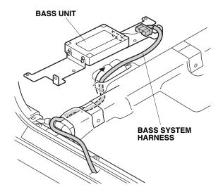
23. Secure the bass system harness to the bass unit using two EPT sealers.
