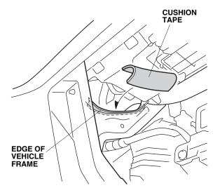
30. Route the bass system harness along the vehicle frame towards the center of the vehicle.
