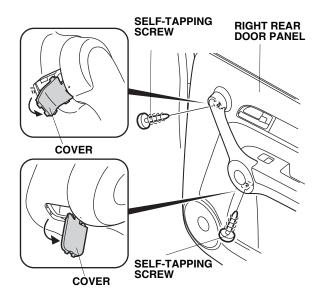
38. Pull the right rear door panel out toward you to release the seven clips, remove the inside handle from the door panel (three clips), disconnect the vehicle connector, and remove the right rear door panel.
