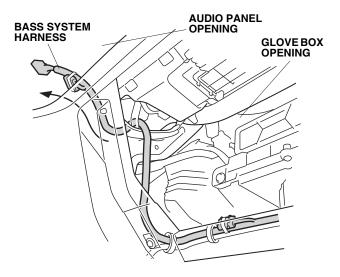
33. Connect the bass system harness 17-pin connector to the vehicle 17-pin connector. Secure the connector to the vehicle harness using one wire tie.
