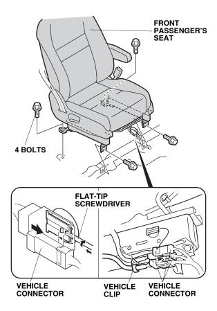
19. Remove the front passenger's seat bolts and tilt the front passenger's seat back (four bolts and vehicle connectors).
