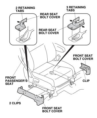
17. Remove the front seat bolt covers from the front passenger's seat (three clips).
