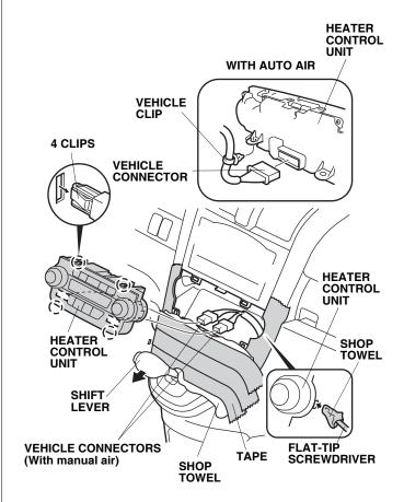
9. Using a flat-tip screwdriver wrapped with a shop towel, remove the heater control unit (four clips and disconnect the vehicle connector(s).
