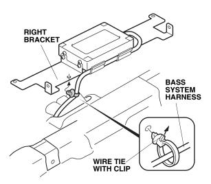
25. Install the bass unit to the front passenger's seat frame using four 5 x 12 mm washer-bolts and four 5 mm flange nuts.
