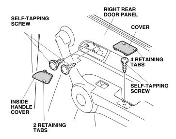
36. Remove the cover (four retaining tabs) and remove the self-tapping screw from the right rear door panel.
