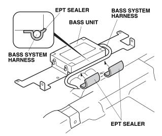
24. Secure the bass system harness to the right bracket using one wire tie with clip.
