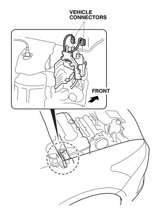
10. Release the vehicle harness holder from the vehicle bracket (two hooks).
