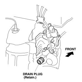
12. Install the engine block heater with the aluminum washer into the engine block using a 24 mm socket and a 100 mm extension. Torque the engine block heater to 60 N·m (44 lb-ft). Using an extension longer than 100 mm will give you an incorrect torque.
