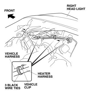
20. Route the heater harness as shown, and secure the wire tie with clip (point G) to the vehicle frame.
