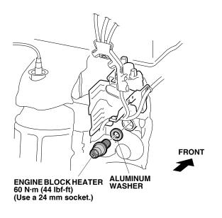
13. Plug the connector on the heater harness into the engine block heater. Route the heater harness as shown, and secure the two wire ties with clips (points A and B) to the vehicle bracket.
