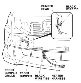
24. Attach the protective cap to the front bumper grille, and plug the connector of the heater harness into the protective cap.
