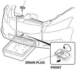
6. Remove the vehicle bracket (one vehicle bolt).
