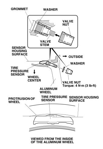
7. While holding the tire pressure sensor to keep it from rotating, torque the valve nut to 4 N·m (0.4 kgf·m, 3 lbf-ft). You may hear a snap or pop as you torque the nut: this is normal.
